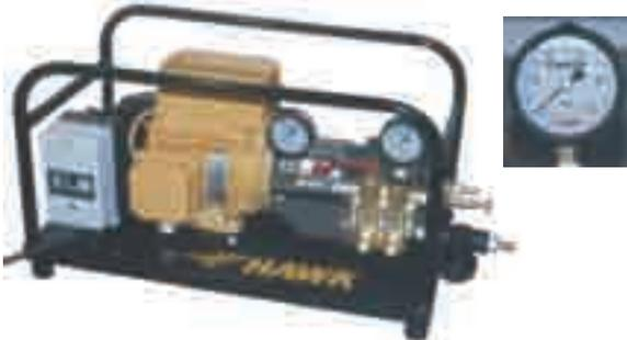
The new Hawk Pressure Testing unit makes testing pipes for leaks a simple operation. Simply plug the one end of the pipe, fill it with water and connect the unit to the other end. Then increase the pressure in the pipe and watch the gauge. If the pressure drops
