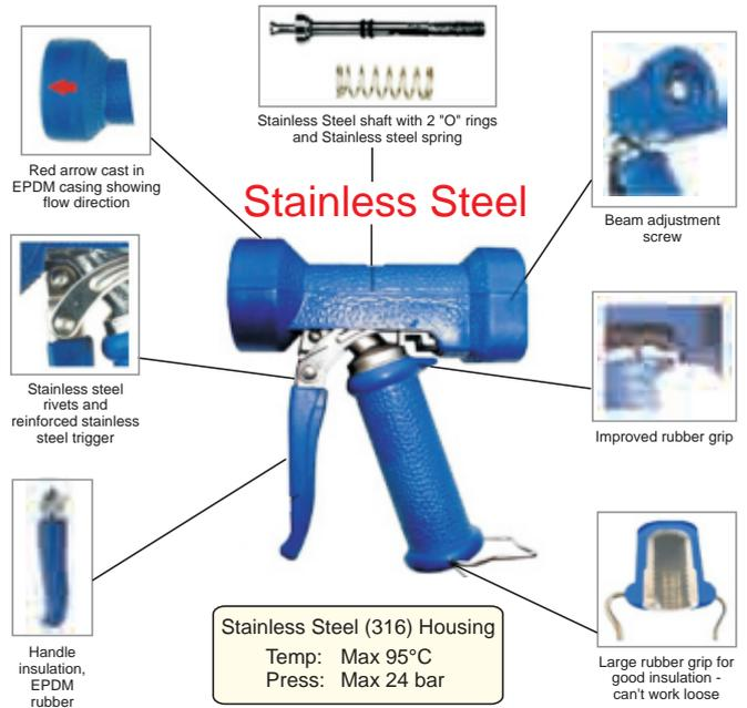
The industrial water gun is a heavy-duty item available with a brass, chrome plated brass, or a full stainless steel (316) body. It has stainless steel rivets, insulated stainless steel trigger handle, reinforced trigger and a robust blue or white EPDM rubber casing for impact protection. The water pattern is adjustable from a fine spray to concentrated jet.
