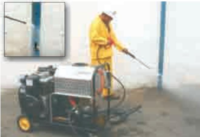
The Hawk unit pictured here is a new version. Using a 17kW diesel engine with electrical start, this machine produces 21 L/min at 350 bar.
