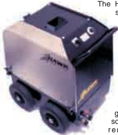
The Hawk Hotbox is the ideal solution for companies who need to add hot water as an option to existing cold water high pressure cleaners. It is fitted between your cold water machine and your high pressure gun and lance and heats the water to a scorching 90°C. This is incredibly useful for applications where heavy grease and other non water-soluble grime needs to be removed. Another key advantage is that you can
