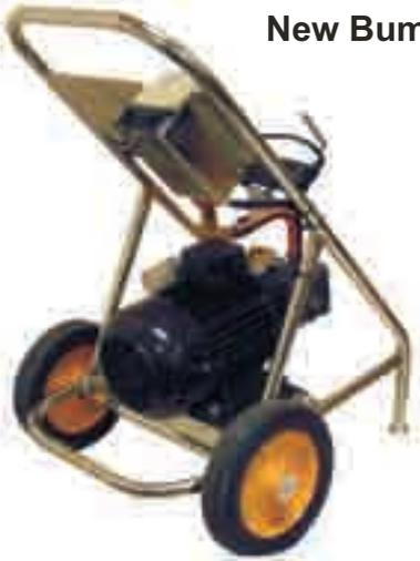
We have improved our standard electric high pressure cleaner chassis by adding a bumper. It helps to protect the motor from being knocked and damaged. Another advantage of this innovation is for lifting the unit for loading.
