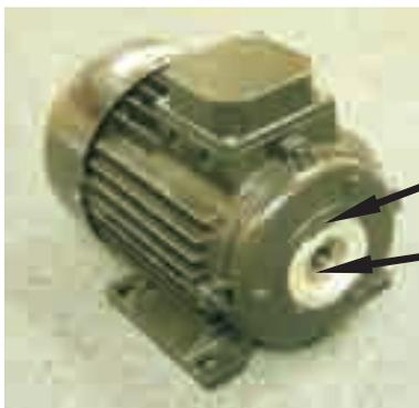
Large bearing supports the front end of the hollow-shaft rotor
