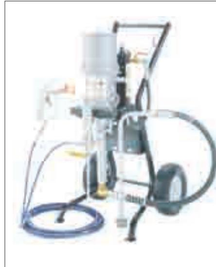
These sprayers deliver trouble free reliability, mainly because of the slow piston stroke rate (a maximum of 60 strokes per minute), and because of the fact that they are made from stainless steel. In addition to the new 40:1 range arriving later this month, we are still able to supply the Graco President 30:1 (paint pressure of up to 210bar)
