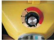
Regulating valve to adjust droplet size
